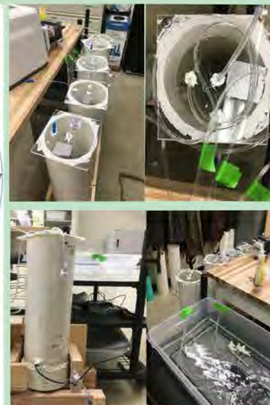
Figure 4 - The picture in the top left depicts all the columns. The top right depicts a top view of one of the columns, which has a plexiglass lid with holes for inflow/outflow/sampling. The bottom left picture shows a side view of a column. The bottom right picture shows the reservoir that all the columns receive their inflow water from and eventually outflow into.
